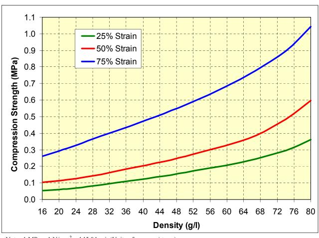
Note: 1 MPa = 1 N/mm<sup>2</sup> = 145.04 psi (Units of pressure/stress) Tested per ASTM-D3575
