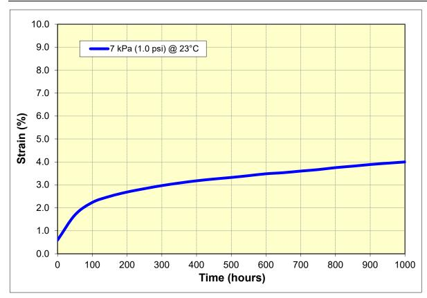
Note: 20 g/l = 1.3 pcf = 45X (g/l = grams per liter; pcf = pounds per cubic foot; X = foam expansion ratio) Tested at 7 kPa (1.0 psi) Tested at Ambient Conditions: 23°C ±3°C (73°F ±5°F) Tested per ASTM D3575
