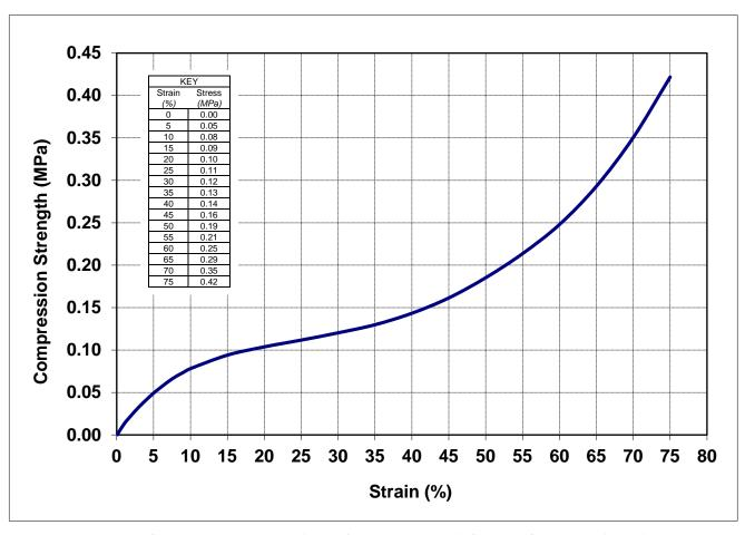
Note: 37 g/l = 2.3 pcf = 25X (g/l = grams per liter; pcf = pounds per cubic foot; X = foam expansion ratio) 1 MPa = 1 N/mm<sup>2</sup> = 145.04 psi (Units of pressure/stress) Test Speed at 12.5 mm/minute (per ASTM-D3575)
